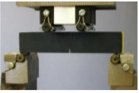
Run past specimen failure and continue to run until the load *returns* to around (-)0.3 kN.
