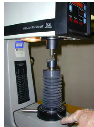
Figure 3. Compression specimen in a Rockwell hardness tester.
