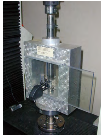
Figure 16. Center the Fixture on the Instron machine platen.
