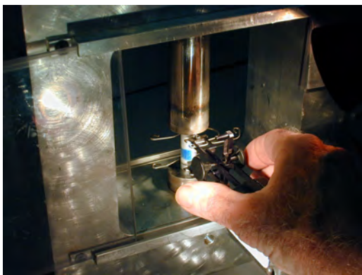
Figure 13. Carefully release the extensometer buttons.
