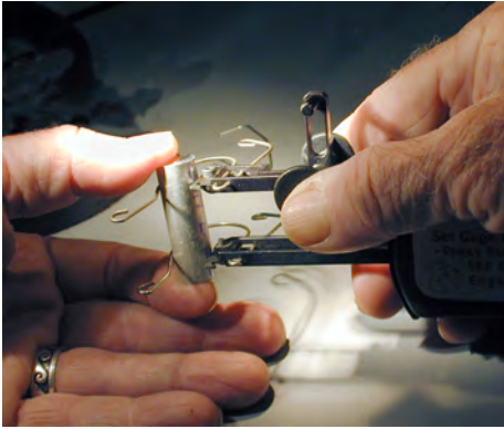
Figure 9. Center the specimen in the clips.
