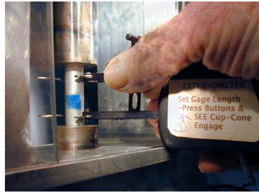
Figure 12. Lower the piston to contact the specimen.
