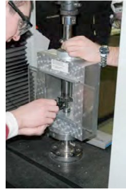
Figure 10. Have a friend raise the piston.
