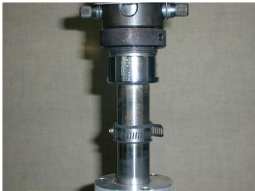
Figure 17. Jog down. Leave a small gap between the platen and the piston.
