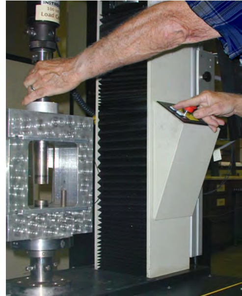
Figure 7. Jog for clearance.
