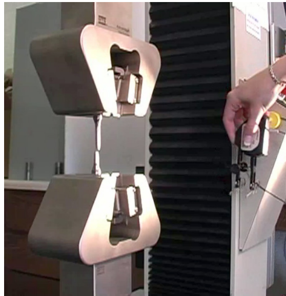
Figure 13. Place the extensometer on its hanger.
